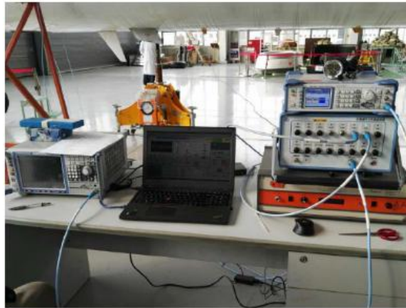
Figure 5: The actual connection diagram of the front door test system.
